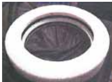
Emergency Custom Fabricated Bushing Clamp
