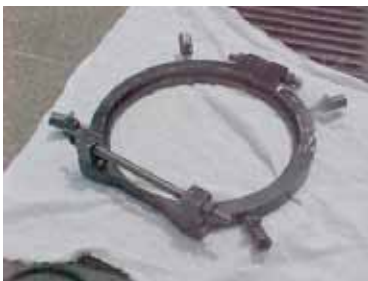
Emergency Custom Fabricated Bushing Clamp
